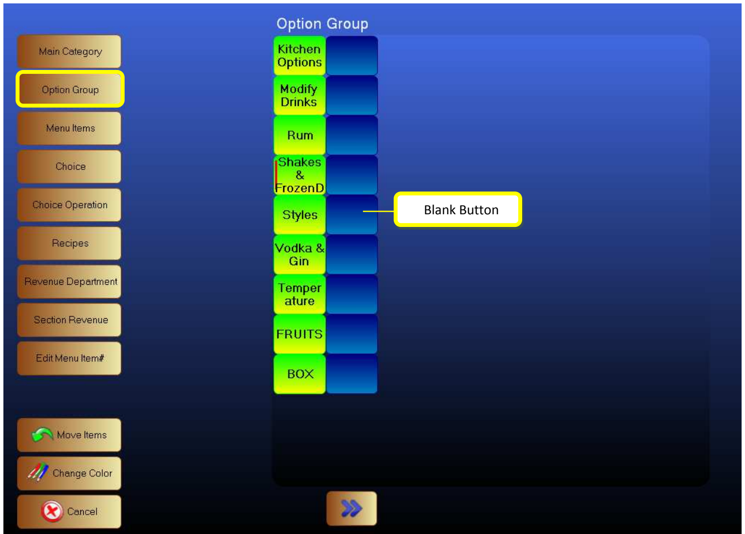
Figure 4 1. Login to Back Office click on Menu then Option Group 2. Create an Option Group by clicking on an Empty Button under option group. This will bring you to the option group setup screen. (Figure 7)
